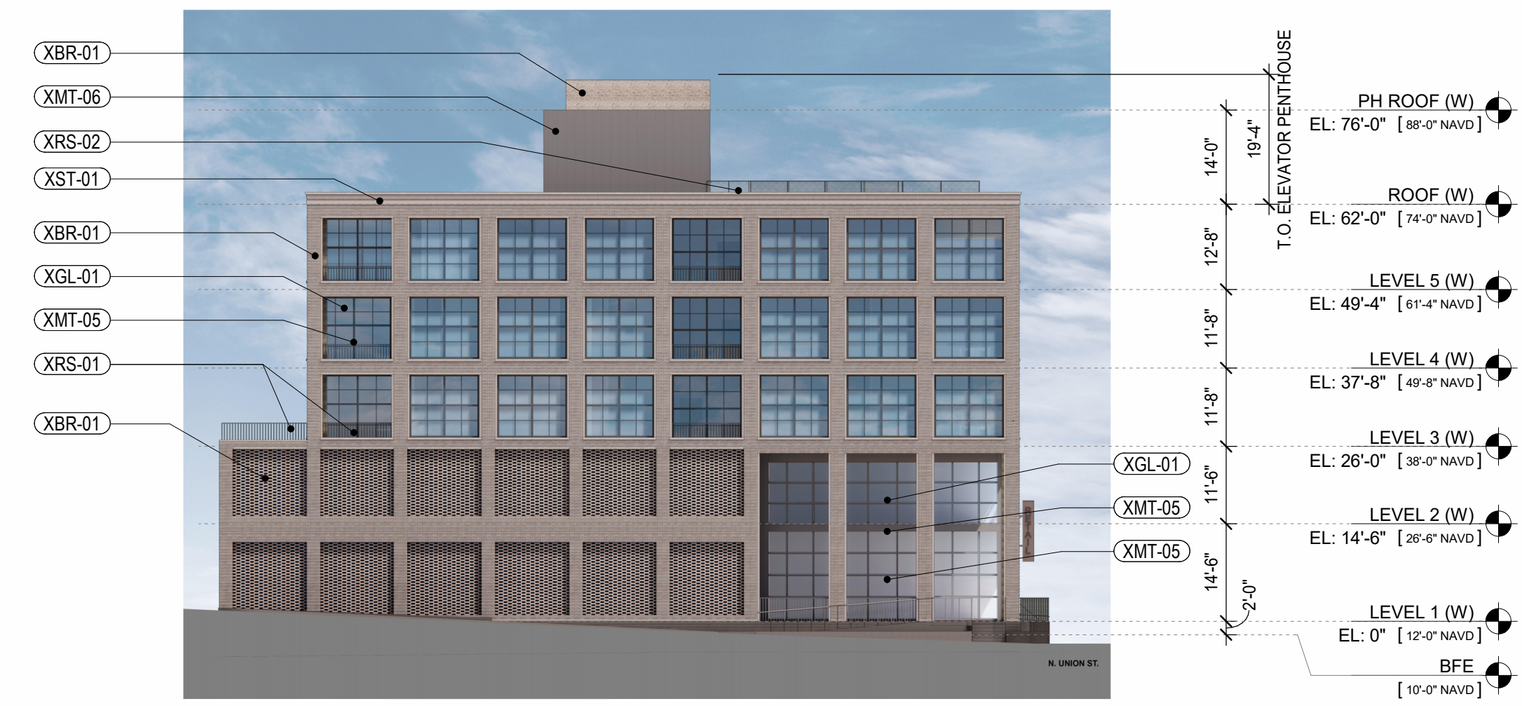
3 BUILDING 500, ELEVATION - SOUTH 1" = 20'-0"
