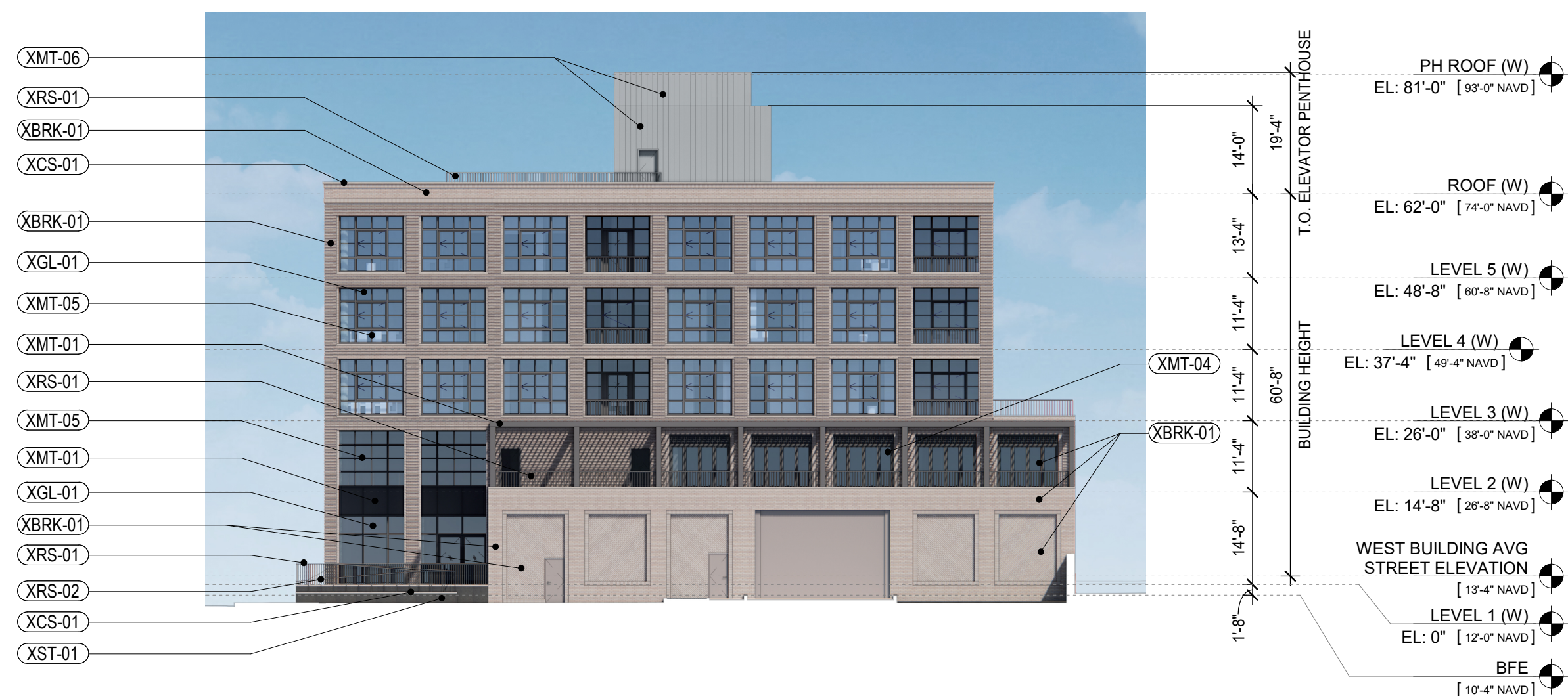
4 BUILDING 500, ELEVATION - NORTH 1" = 20'-0"
