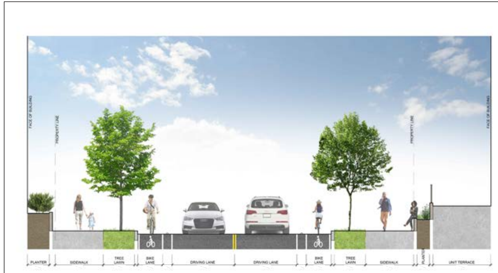
1 N. UNION STREET TYPICAL SECTION L501 SECTION
